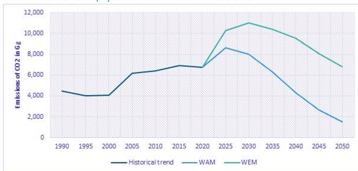
Figure 2.26: Historical trends of CO 2 emissions in Gg from road transport for the years 1990 – 2020 and emission projections in the WEM and WAM scenarios
