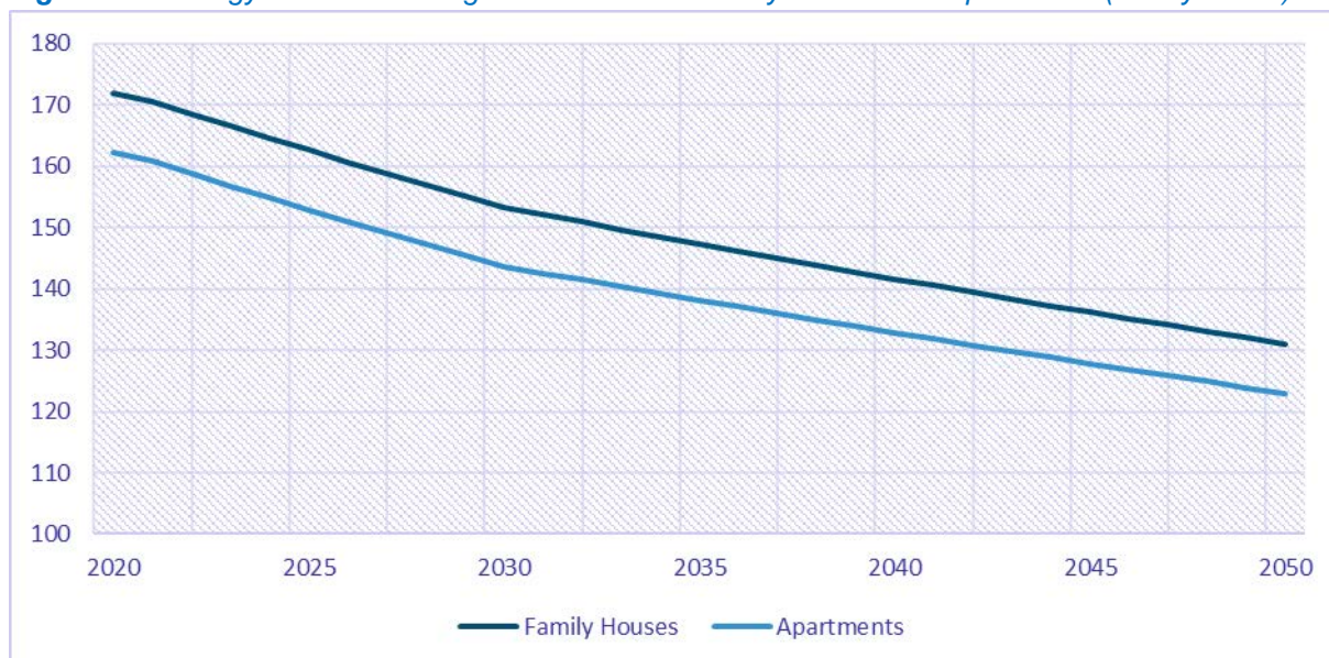
Figure 2.2: Energy need for heating and hot water in family houses and apartments (kWh/year/m 2 )
